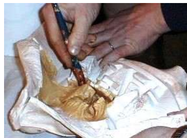
Put by brush some Acrystal on the mould sides to prevent getting bubbles on the surface.
